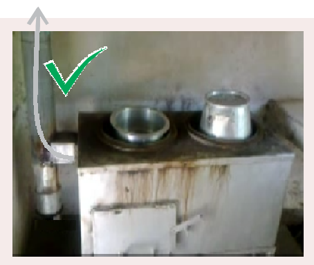
Improved kitchen whereby all the smoke goes out through the chimney This improved kitchen is also fuel-efficient and consumes less firewood.
